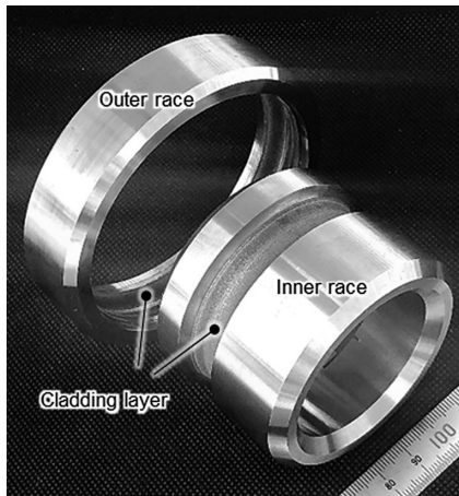
Fig. 14 Appearance of inner and outer race cladding by non-molten pool LMD.
