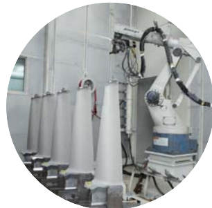
Thermal spraying onto turbine blades
