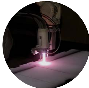
Plasma spraying onto carbon sheets
