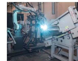
Automatic welding using robots
