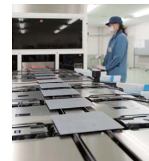
Inspection of all products using an automated inspection machine
