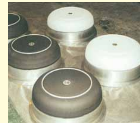
- Induction heating pot : size \Phi 550 \times 250 H
