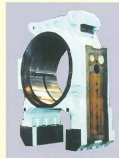
- Backup roll chuck : size : 1700x1100x2700(38ton )
