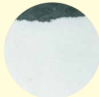
Spraying material : tungsten carbide cobalt (200 magnifications)
